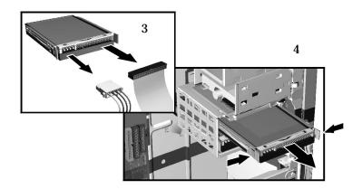
5. Remove the two blue guide rails by gently prying them off the hard disk drive. These guide rails will be required for the new disk drive.
